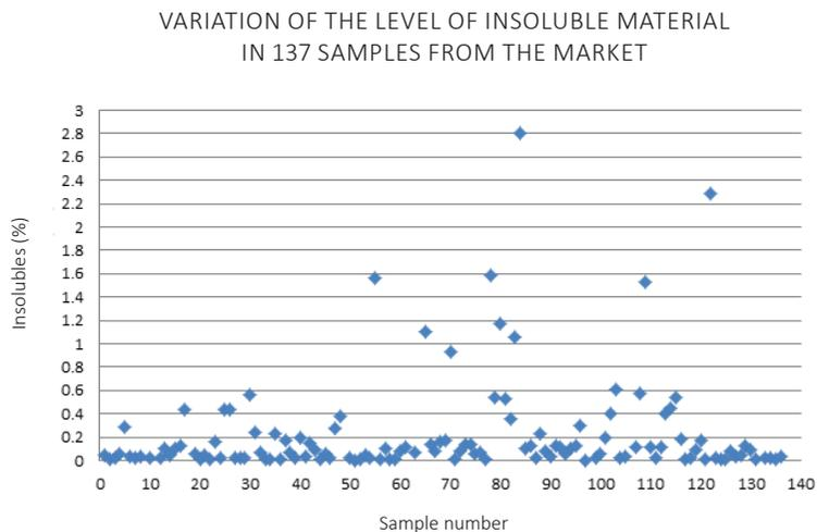
Figure 5: Content of insolubles in 137 SOP samples
