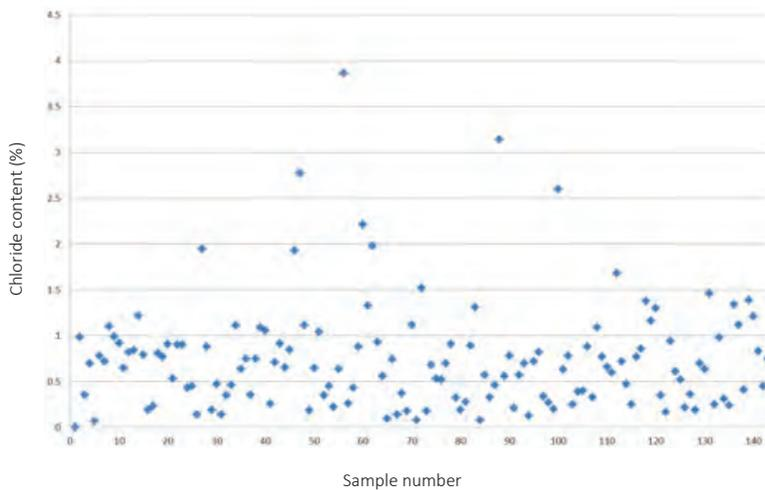
Figure 3: Chloride content in 143 SOP samples
