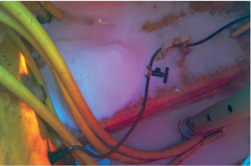
*Results from an 8 % solution after spraying - much of the product did not dissolve and remains in the tank*
