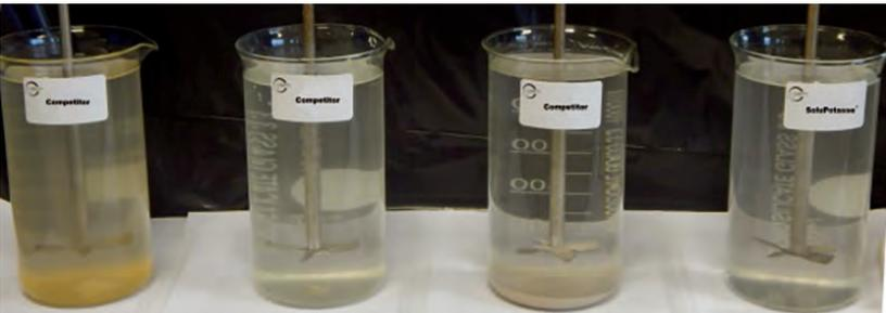
Figure 1: Different samples in solution, compared to SoluPotasse as the rightmost reference sample on the pictures (left after 1 minute of stirring; right after 15 minutes of stirring); (Tests shown were conducted using de-ionised water for consistency)
