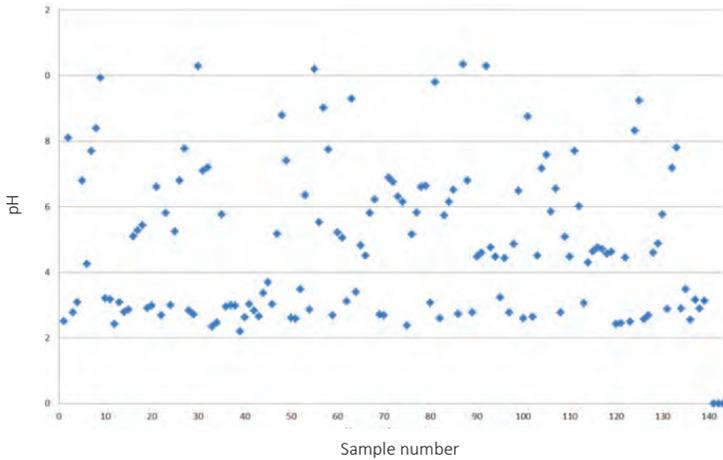
Figure 6: pH at 1 % in 143 SOP samples
