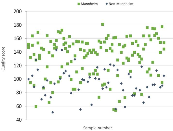
Graph 2: QI of soluble SOP samples per production process
